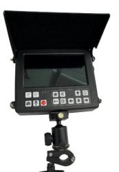
1. POWER Press the button for 3 seconds to turn on /off the control box
