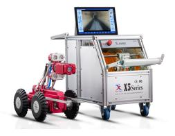
X5-HS pipeline CCTV Inspection robot is Easy Sight' the fourth generation product designed on the basis of industrial personal computer (IPC) system, using a laptop instead of the traditional controller.
